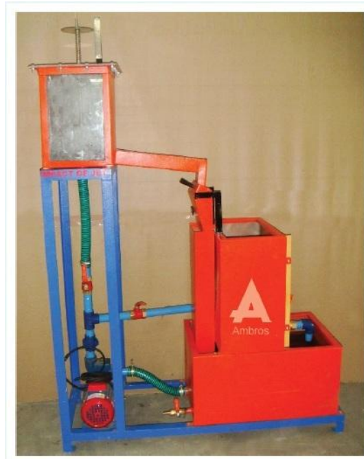
Figure 5.1 Impact of Jet on Vanes Apparatus
