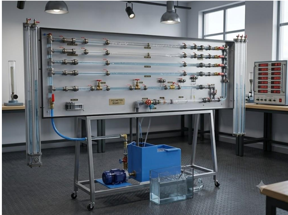
Figure 4.1 Determination Of Friction Apparatus
