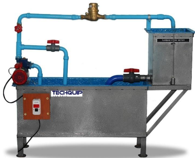
Fig 2 Experimental Setup for testing the Turbine Flow Meter
