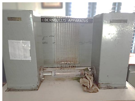
Figure 1.2(b): Bernoulli's Apparatus
